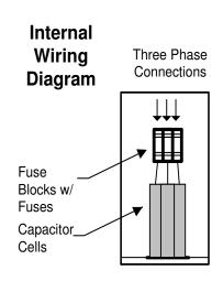
MODEL M002.0-240-F 2.0 KVAR 240 VOLT Fused Three Phase 60 Hz NEMA 3R Enclosure Rated Current: 4.8 Amps Recommended Wire Size: 14 AWG
