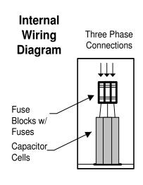
MODEL M011.0-240-F 11 KVAR 240 VOLT Fused Three Phase 60 Hz NEMA 3R Enclosure Rated Current: 26.5 Amps Recommended Wire Size: 8 AWG
