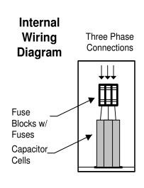
MODEL M012.0-240-F 12 KVAR 240 VOLT Fused Three Phase 60 Hz NEMA 3R Enclosure
