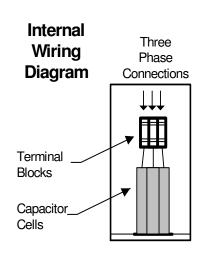
MODEL M016.0-480-NF 16.0 KVAR 480 VOLT Non Fused Three Phase 60 Hz NEMA 3R Enclosure Rated Current: 19.2 Amps
