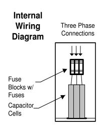
MODEL M016.0-480-F 16.0 KVAR 480 VOLT Fused Three Phase 60 Hz NEMA 3R Enclosure Rated Current: 19.2 Amps Recommended Wire Size: 10 AWG
