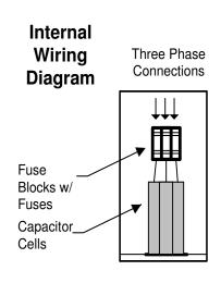
MODEL M018.0-480-F 18.0 KVAR 480 VOLT Fused Three Phase 60 Hz NEMA 3R Enclosure
