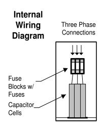
MODEL M026.0-480-F 26 KVAR 480 VOLT Fused Three Phase 60 Hz NEMA 3R Enclosure Rated Current: 31.2 Amps Recommended Wire Size: 6 AWG
