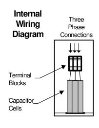
MODEL M026.0-480-NF 26 KVAR 480 VOLT Non Fused Three Phase 60 Hz NEMA 3R Enclosure Rated Current: 31.2 Amps Recommended Wire Size: 6 AWG APPROX. WEIGHT 30 LBS. EACH
