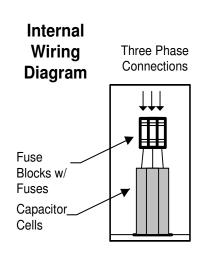
MODEL M027.5-480-F 27.5 KVAR 480 VOLT Fused Three Phase 60 Hz NEMA 3R Enclosure Rated Current: 33.1 Amps
