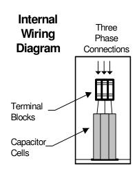
MODEL M027.5-480-NF 27.5 KVAR 480 VOLT Non Fused Three Phase 60 Hz NEMA 3R Enclosure Rated Current: 33.1 Amps
