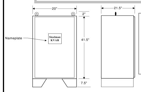
**Life Expectancy:** 20 years **Temperature:** -40°C to +50°C **Discharge Resistors:** Included, will reduce residual voltage to less than 50 yolts in one minute after removal
