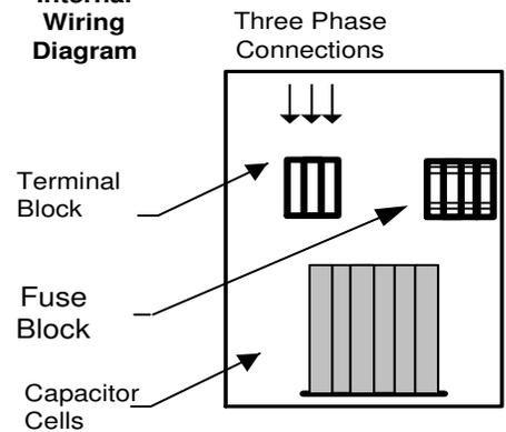
Enclosures are rated NEMA 1, Indoor. Designed to be floor mounted. Lifting eye bolts on all Pad-Mount Units. Electrical Connections should be made through the top right.
