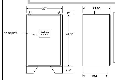
**Life Expectancy:** 20 years **Temperature:** -40°C to +50°C **Discharge Resistors:** Included, will reduce residual voltage to less than 50 volts in one minute after removal from service.
