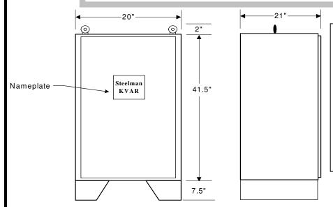
**Life Expectancy:** 20 years **Temperature:** -40°C to +50°C **Discharge Resistors:** Included, will reduce residual voltage to less than 50 volts in one minute after removal from service.
