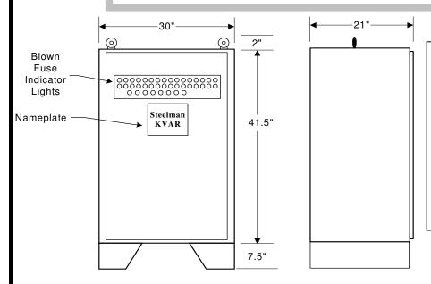
**Life Expectancy:** 20 years **Temperature:** -40°C to +50°C **Discharge Resistors:** Included, will reduce residual voltage to less than 50 volts in one minute after removal
