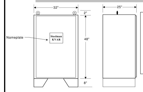
**Life Expectancy:** 20 years **Temperature:** -40°C to +50°C **Discharge Resistors:** Included, will reduce residual voltage to less than 50 volts in one minute after removal from service.
