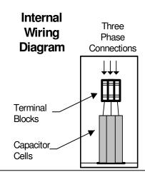
MODEL M009.0-240-NF 9.0 KVAR 240 VOLT Non Fused Three Phase 60 Hz NEMA 3R Enclosure
