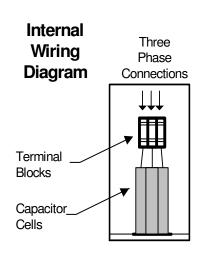
MODEL M022.0-480-NF 22.0 KVAR 480 VOLT Non Fused Three Phase 60 Hz NEMA 3R Enclosure Rated Current: 26.5 Amps
