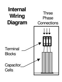
MODEL M023.0-480-NF 23 KVAR 480 VOLT Non Fused Three Phase 60 Hz NEMA 3R Enclosure
