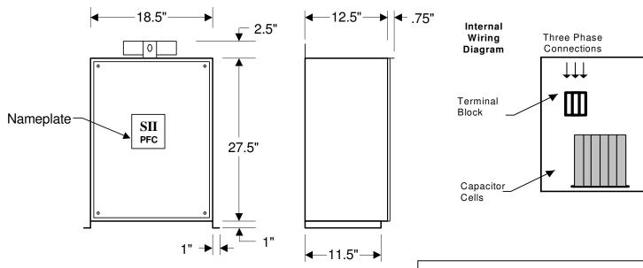
MODEL M040.0-240-NF 40 KVAR 240 VOLT Non Fused Three Phase 60 Hz NEMA 3R Enclosure Rated Current: 96.2 Amps Recommended Wire Size: 1 AWG
