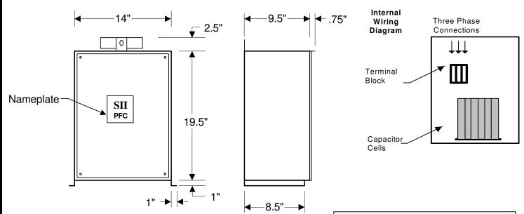
MODEL M055.0-480-NF 55 KVAR 480 VOLT Non Fused Three Phase 60 Hz NEMA 3R Enclosure Rated Current: 66.2 Amps
