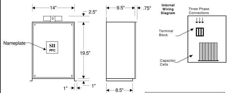
MODEL M060.0-480-NF 60 KVAR 480 VOLT Non Fused Three Phase 60 Hz NEMA 3R Enclosure Rated Current: 72.2 Amps
