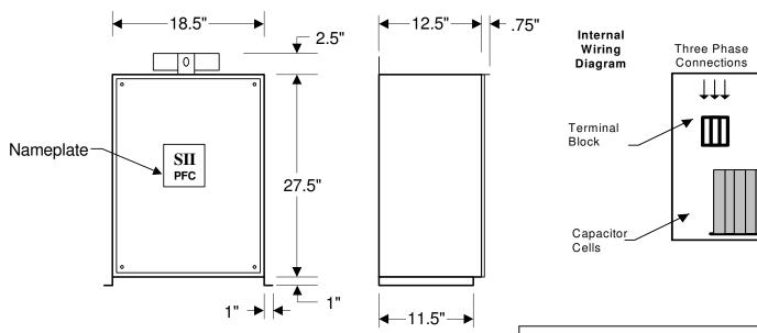
MODEL M090.0-480-NF 90 KVAR 480 VOLT Fused Three Phase 60 Hz NEMA 3R Enclosure Rated Current: 108.3 Amps Recommended Wire Size: 1/0 AWG
